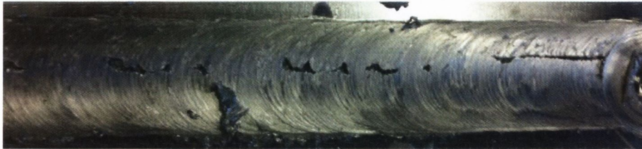
Figure 214: Surface defects due to a high translational speed 355mm/min
