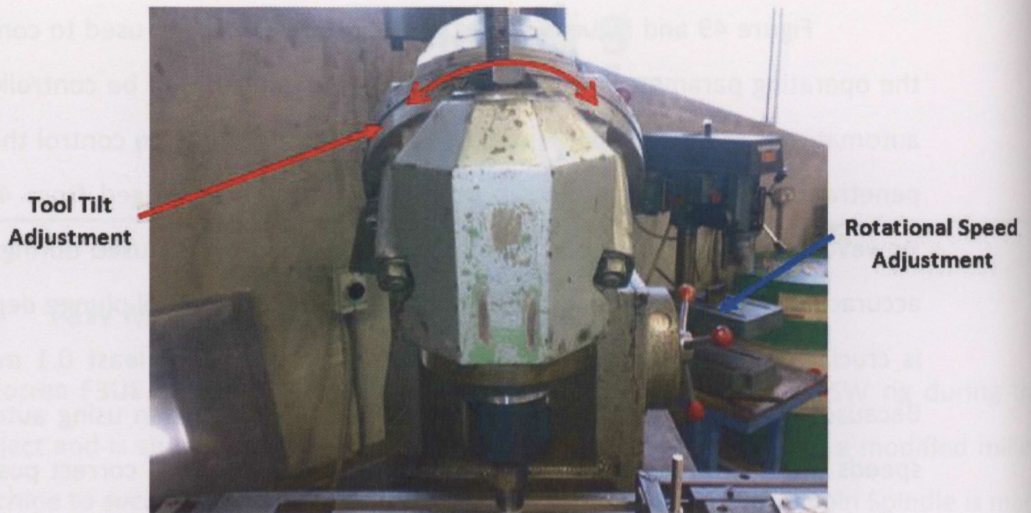
Figure 50: Rotational speed and tool tilt angle adjustment
