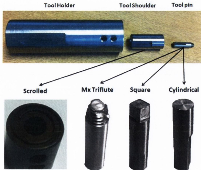
Figure 198: FSW tooling, shoulder and pin designs.
