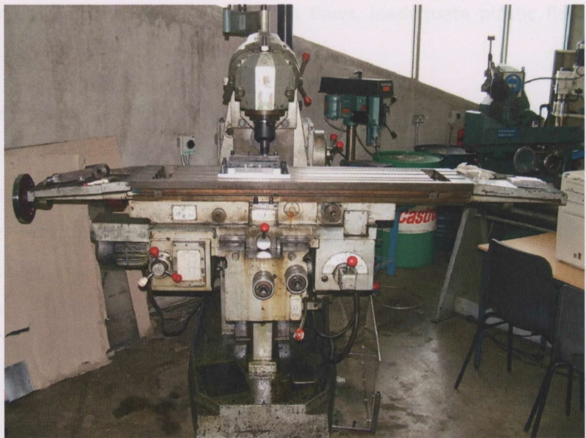
Figure 48: Modified milling machined converted to perform FSW at Trinity College Dublin
