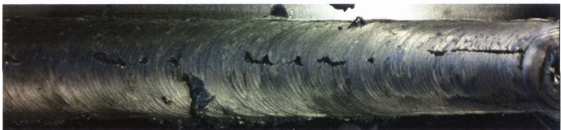
Figure 126: Surface defects due to a high translational speed
