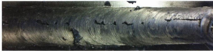
Figure 203: Surface defects at 500mm/min translational speed.
