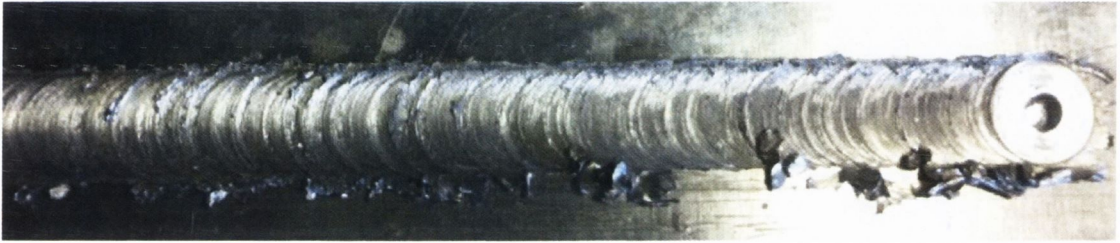
Figure 59: Bad surface finish from scrolled design A with 2° tilt angle
