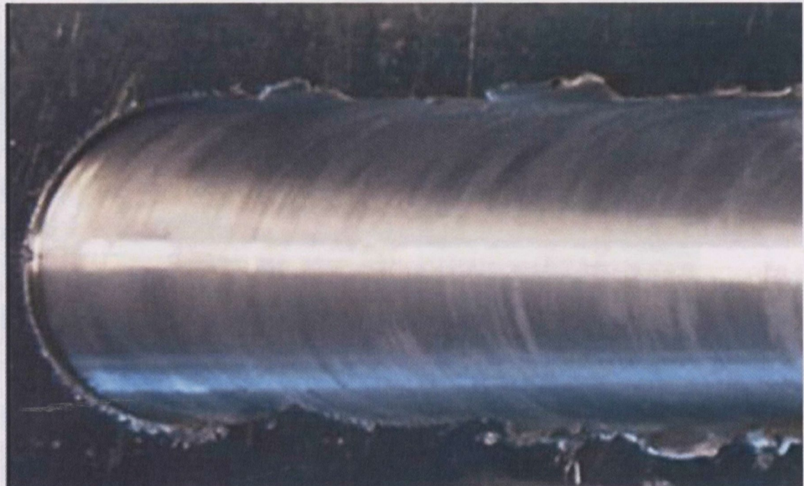
Figure 76: Smooth surface finish with no surface defects
