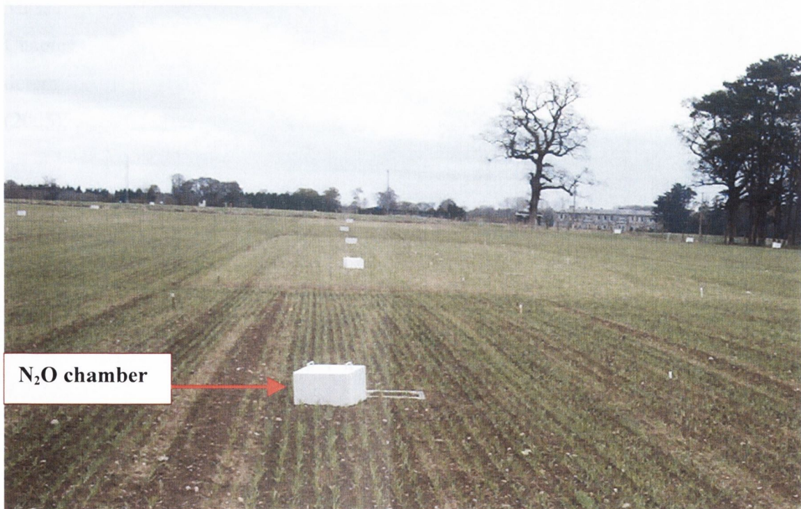
Figure 4.3: Experimental field showing growing barley and installed chambers
