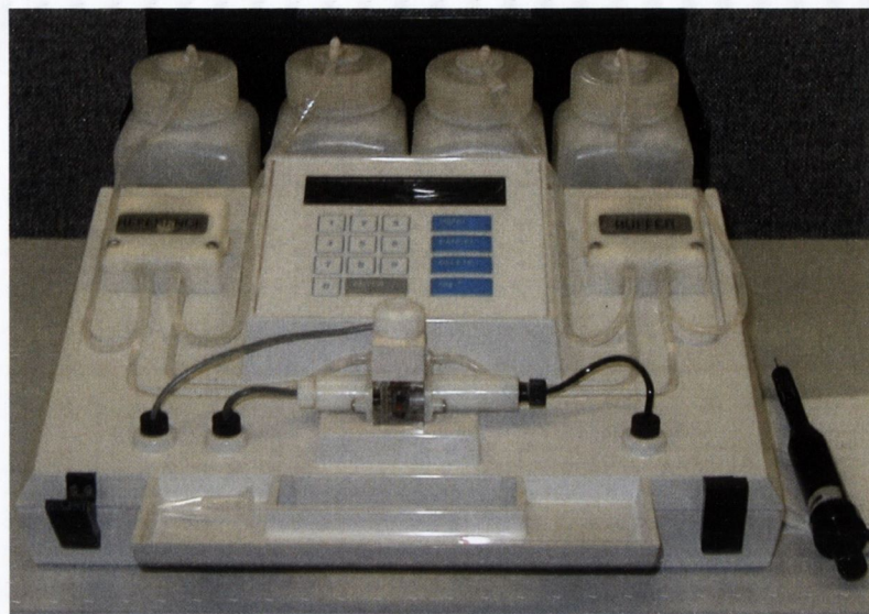
Figure 2.4: YSI 1500 Sport Lactate analyser.
