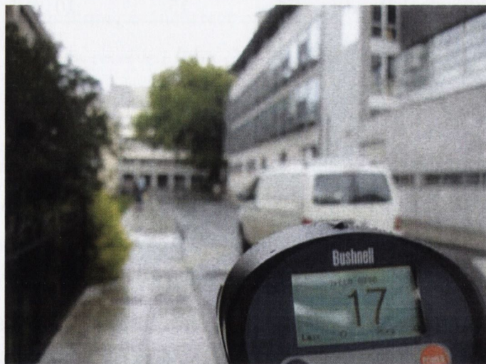
FIGURE 3.1: Determining Traffic Speed by Radar
