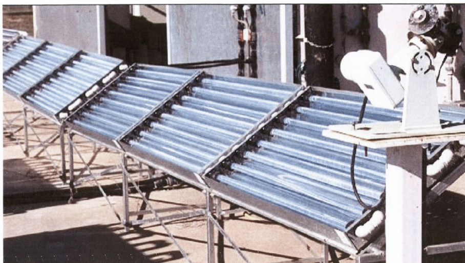
Figure 3.12: Pilot scale reactor located at Plataforma Solar de Almería.
