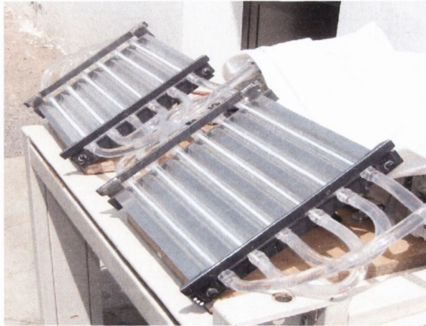
Figure 3.11: Two Small-scale solar disinfection reactors exposed to natural solar radiation at PSA.
