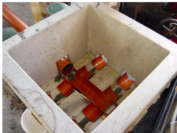
Figure 3.4. Distribution box with V-notch weir modifications in the laboratory.
