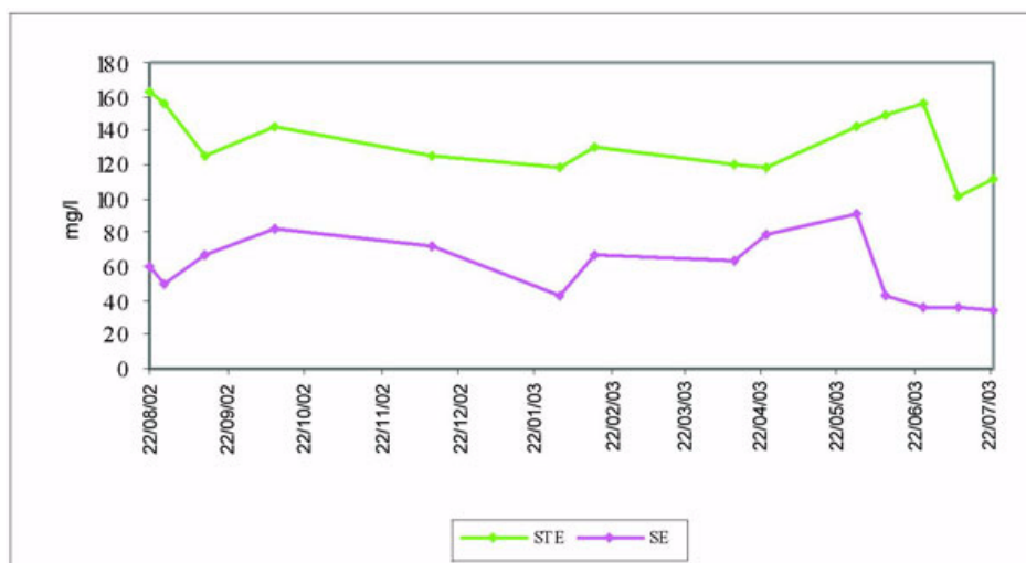
Figure 5.1. Reduction in total inorganic N concentration across the secondary treatment system.
