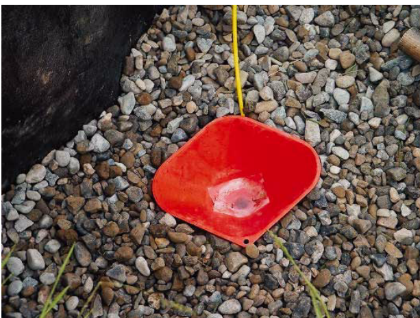
Figure 3.11. Installation of gravity samplers in sand filters.
