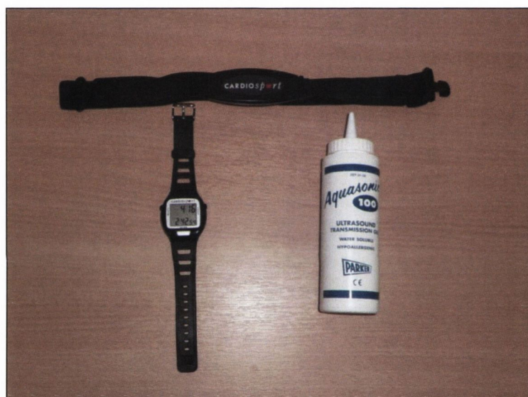
Plate 2.11: CardioSport heart rate monitor and transmitter with ultrasound transmission gel.
