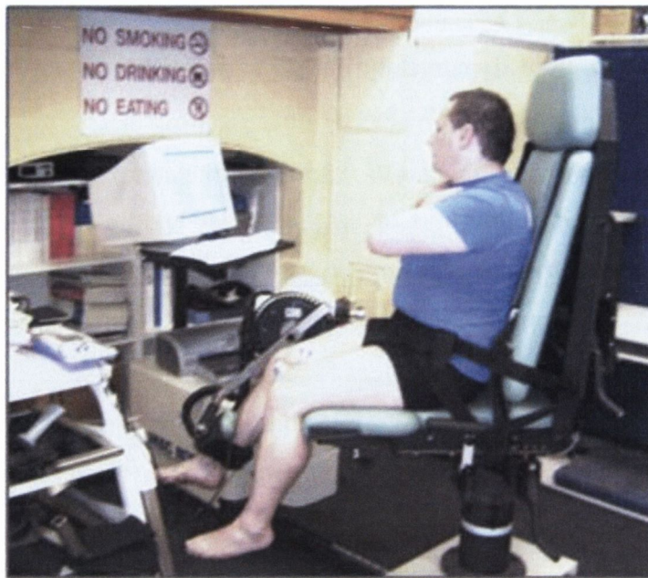
Plate 4.2: Participant performing maximal voluntary isometric knee extensions on the Cybex II dynamometer.
