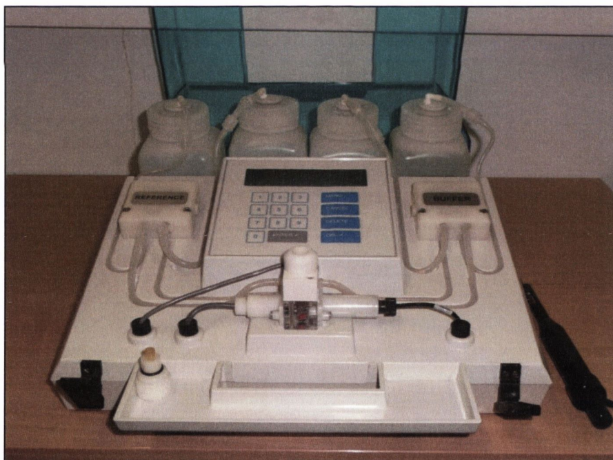
Plate 2.10: YSI 1500 Lactate Analyser with 25\mu\text{L} syringe pipette
