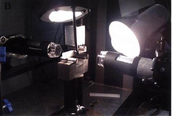
Figure 9.2. Fracture toughness tests set-up for (A) compact tension and (B) single edge notched beam specimen with crack monitoring system.
