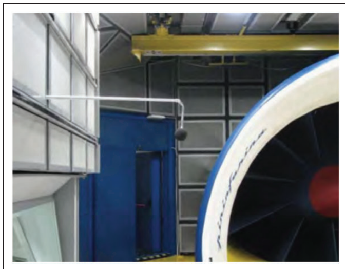
Figure 2. Out-of-flow microphone used for background measurements.
