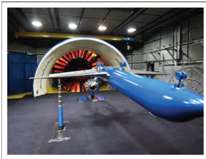
Figure 1. Pininfarina wind tunnel facility with full model installed.
