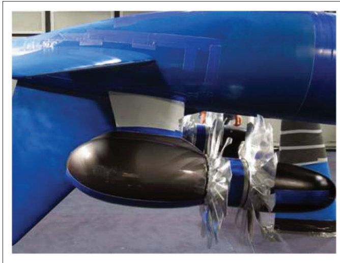
Figure 4. Installed CROR engine in tractor configuration.
