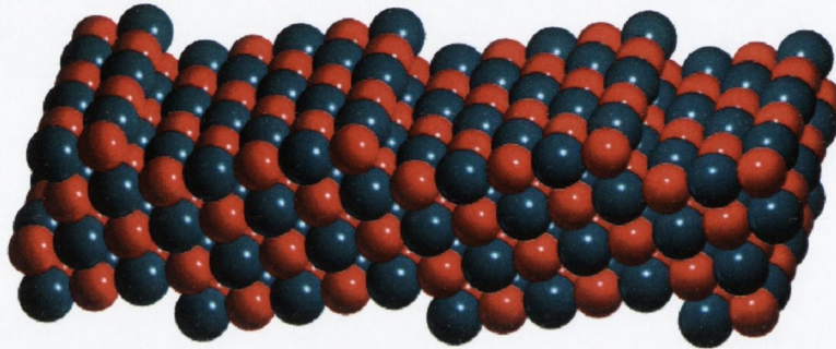
Figure 6.1: High-miscut surface of MgO (miscut angle 11.3^\circ ) shown to the atomic scale. Red and grey spheres represent O and Mg atoms respectively. We note the presence of plateaus of the low-index surface, separated by atomic height steps.
