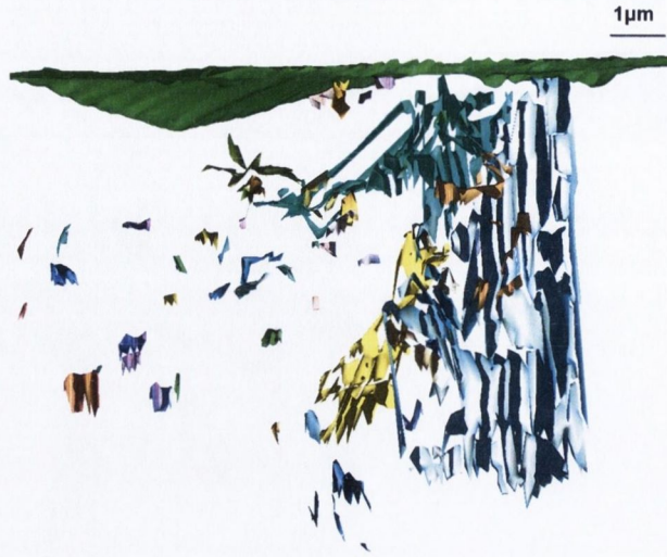
Figure B.4: Side view of a 3D reconstruction of a Vickers indentation at 1 N in Syalon 101.
