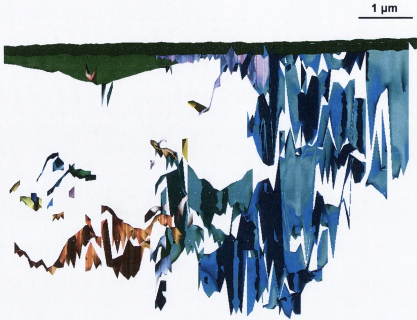
Figure B.20: Side view of a 3D reconstruction of a Vickers indentation at 500 mN in Syalon 050.
