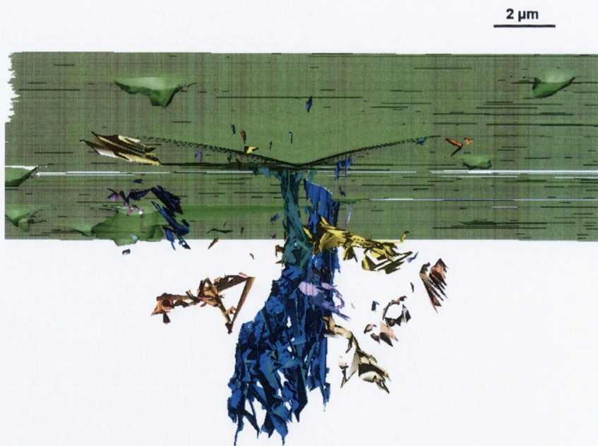
Figure B.21: Top view of a 3D reconstruction of a Vickers indentation at 1 N in Syalon 050.
