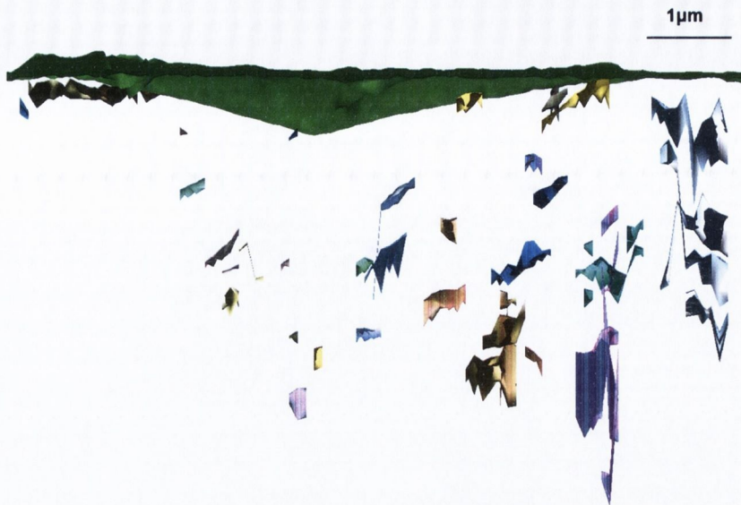
Figure B.2: Side view of a 3D reconstruction of a Vickers indentation at 500 mN in Syalon 101.
