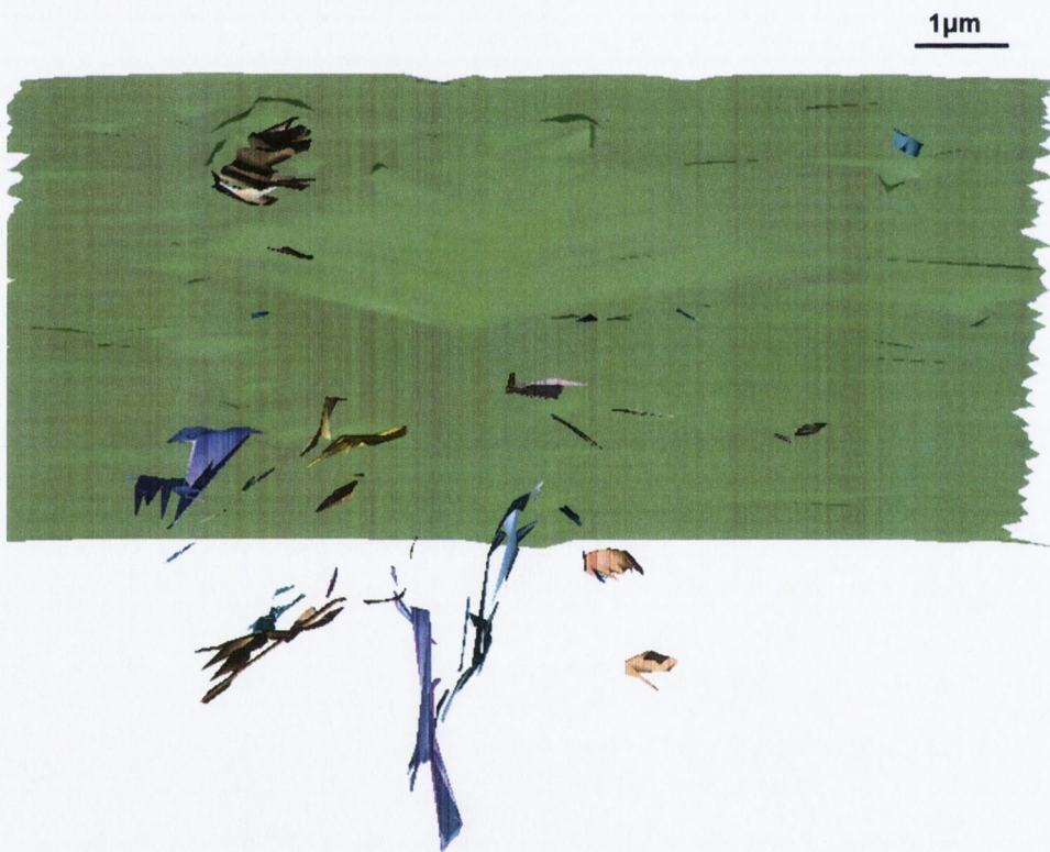
Figure B.1: Top view of a 3D reconstruction of a Vickers indentation at 500 mN in Syalon 101. Each crack has been meshed and is represented with a different color. The surface is in green.
