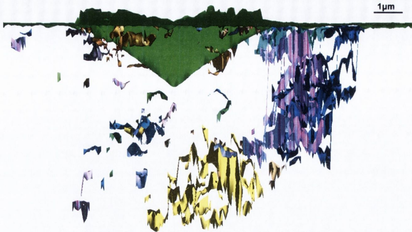
Figure B.14: Side view of a 3D reconstruction of an indentation performed with the customized tip at 500 mN in Syalon 101.
