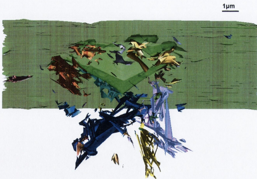
Figure B.13: Top view of a 3D reconstruction of an indentation performed with the customized tip at 500 mN in Syalon 101.
