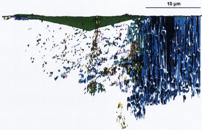
Figure B.12: Side view of a 3D reconstruction of a Vickers indentation at 5N (indent num20) in Syalon 101.
