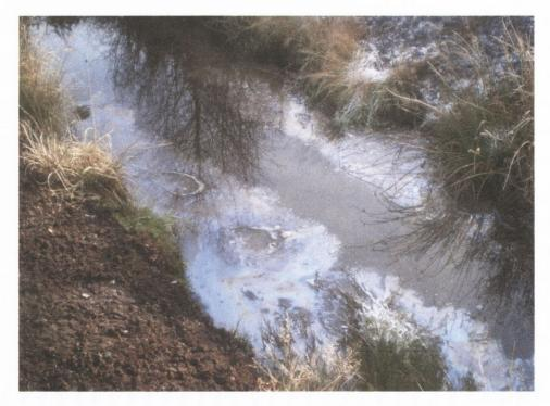
Figure 5.13. Evidence of groundwater discharge at drain FB3, adjacent to piezometer nest 918
