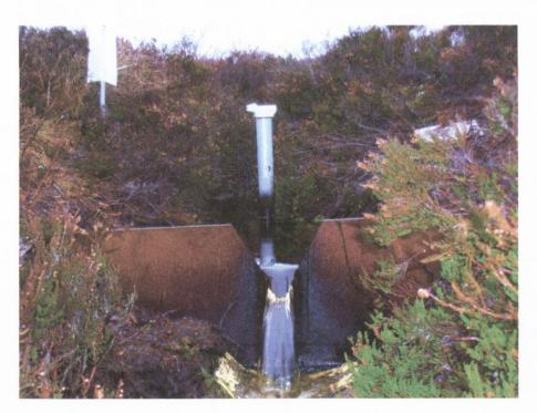
Figure 4.9. High bog v-notch weir and stilling well installed in the Bog Drain
