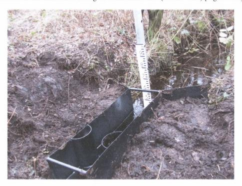
Figure 4.11. Restoration Area Flume installed in Restoration Drain (note: stilling well and staff gauge later moved away from incoming channel stretch to ensure laminar flow).
