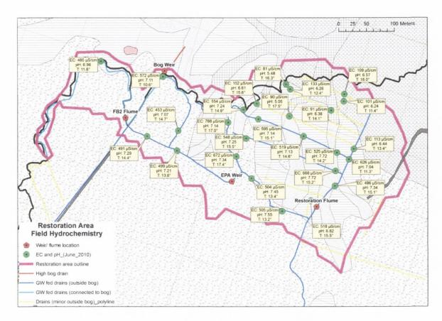
Figure 4.5. Electrical conductivity measurements in drains in Restoration Area, June 2010.
