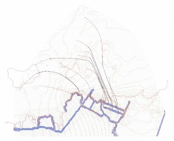
Figure 12.1. Potentiometric surface and flow lines in layer 2 (peat aquifer). Contours are at 0.5 m intervals.
