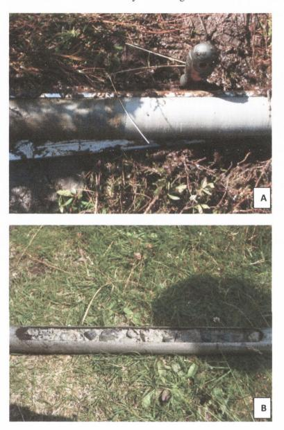
Figure 3.3. (a) Lacustrine clay core from piezometer nest 57. (b) Till core from piezometer 913 (see Appendix C for location map)
