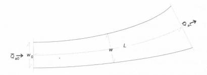
Figure 2.4. Flow path length (L) between two streamlines (Ten Heggler et al, 2004).
