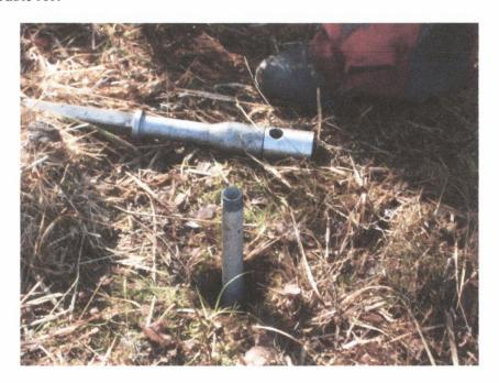
Figure 3.12. Subsoil piezometer 924 - before core-hole is backfilled and sealed.
