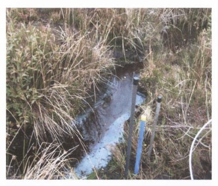
Figure 3.11. Piezometer nest 914 (location: Figure A12; Appendix A) – note iron iridescence in drain
