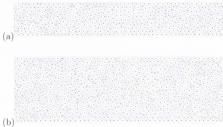
Figure 4.2: Visualisations of two narrow-channel simulations. Packing fraction \phi = 0.98 . (a) L = 8\langle d \rangle , with De = 3.36 \times 10^{-4} , N = 1200 and N_{\text{Wall}}/N = 0.25 . Approximately one third of the channel length is shown. (b) L = 16\langle d \rangle , with De = 1.66 \times 10^{-4} , N = 1380 and N_{\text{Wall}}/N = 0.12 . Approximately two thirds of the channel length is shown.
