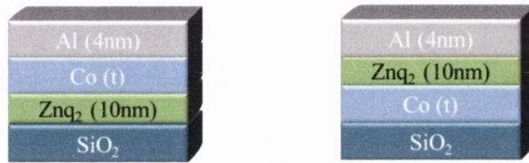
Figure 3.24. The stacks showing that the Co layer is either deposited on SiO 2 or Znq 2 .
