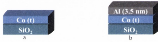
Figure 3.9. The stacks used for magnetic dead layer investigation showing uncapped (a) and capped (b) Co layer.
