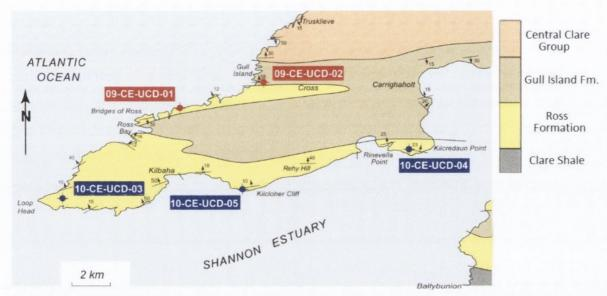
Figure 6.10 Locations of boreholes cored as part of the Co. Clare drilling and training initiative. Red: Proof of concept boreholes. Blue: Phase 2 boreholes. Source: (Haughton et al., 2010)
