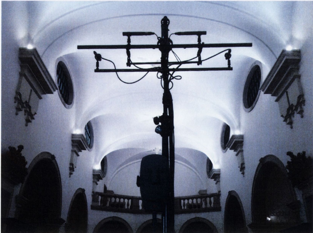
Figure 8-20: Comparative setup for stereo and surround recordings of an orchestra in Aveiro's cathedral, Portugal (front view).
