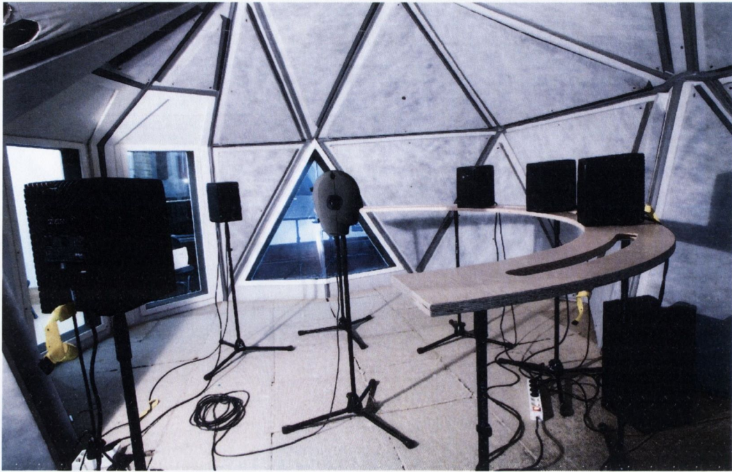
Figure 8-10: IACC measurements of reconstructed sound fields. Serviços de Áudio studio at ESMAE-IPP.
