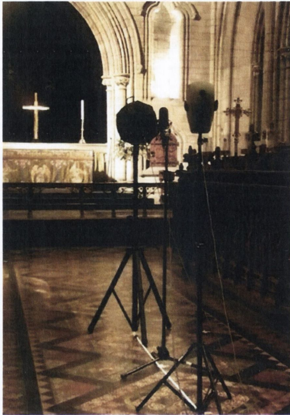
Figure 4.15: Acoustic measurements taken using Brüel & Kjær Omnipower omni-directional source, Soundfield MKV microphone system and Neumann KU-100 binaural microphone
