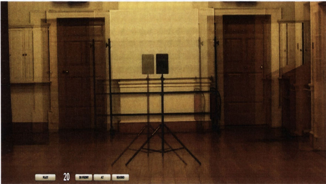
Figure 5.25: Left and right eye views of the stereoscopic image overlaid on top of each other showing a loudspeaker at 4m from the user. Simple GUI was overlaid on top of the image(s) in order to provide means of navigating through the test and saving the results
