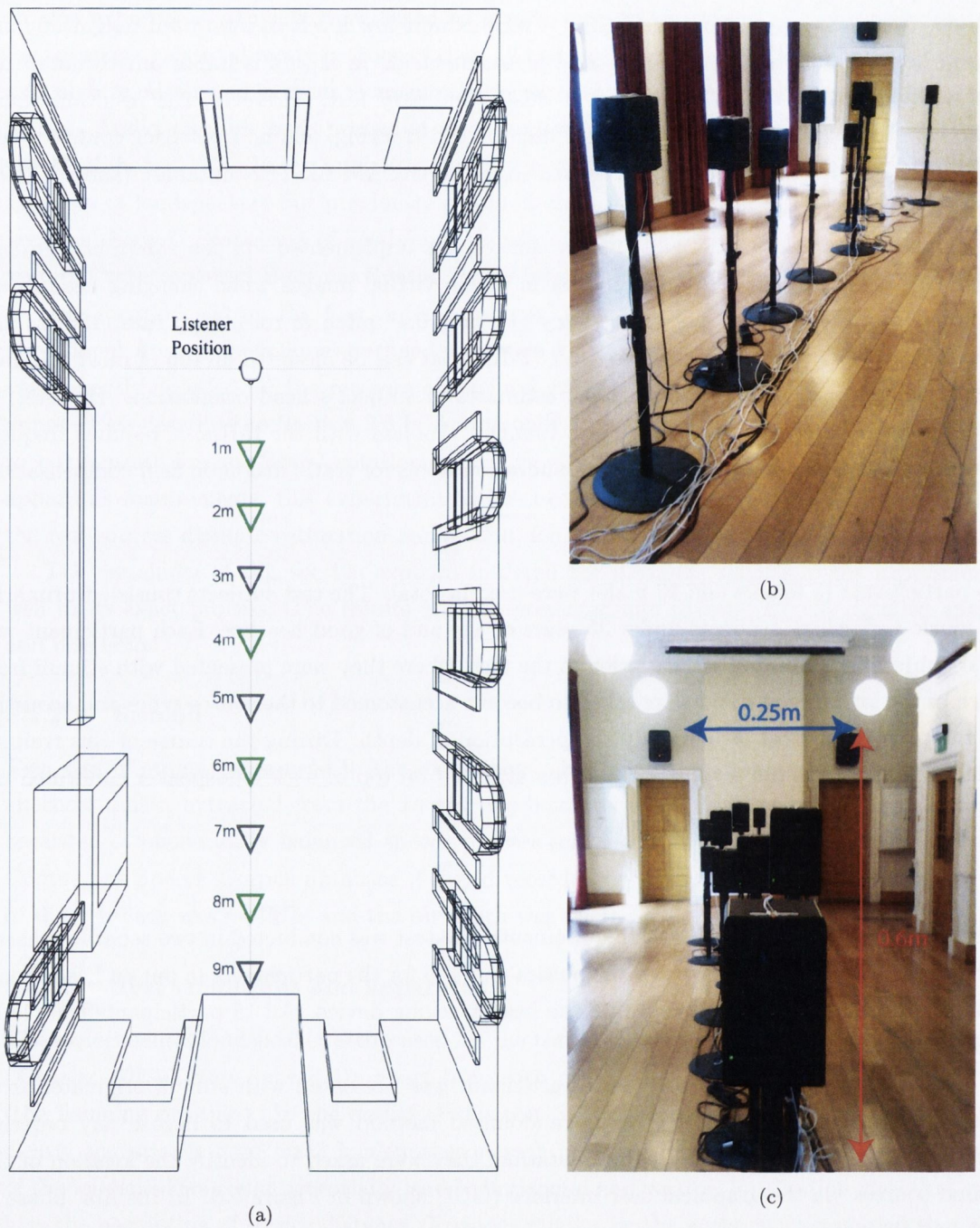
Figure 5.1: Loudspeaker setup for the preliminary distance perception study: (a) Loudspeaker setup diagram; (b) Side perspective of staggered loudspeakers; (c) Subject perspective.
