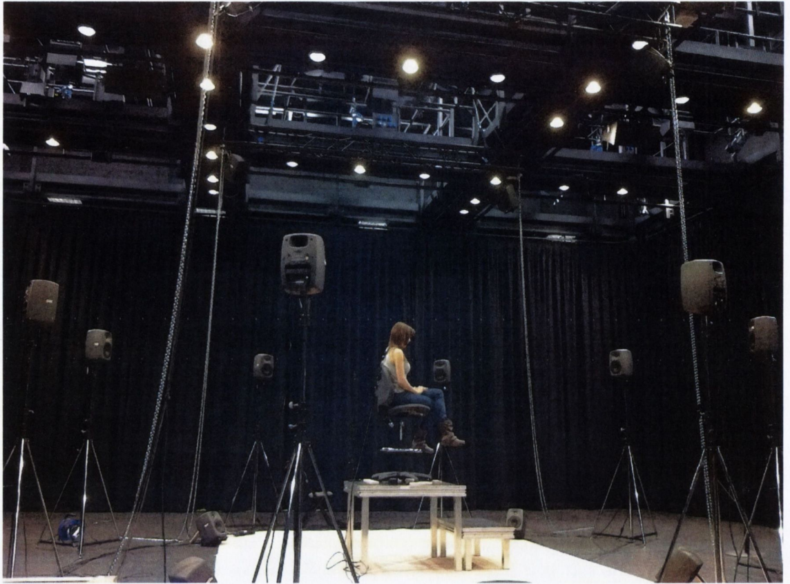
Figure 5.9: Array of 16 loudspeakers used for HRIR measurements
