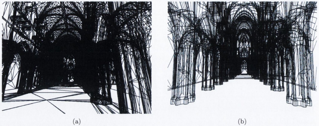
Figure 4.21: Wire-frame model of the church: (a) before polygon reduction process; (b) after polygon reduction process
