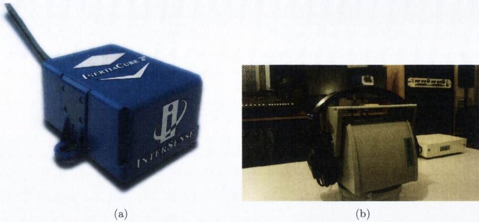
Figure 5.2: Inertial Measurement Unit Intersense InertiaCube2+ used for head tracking
