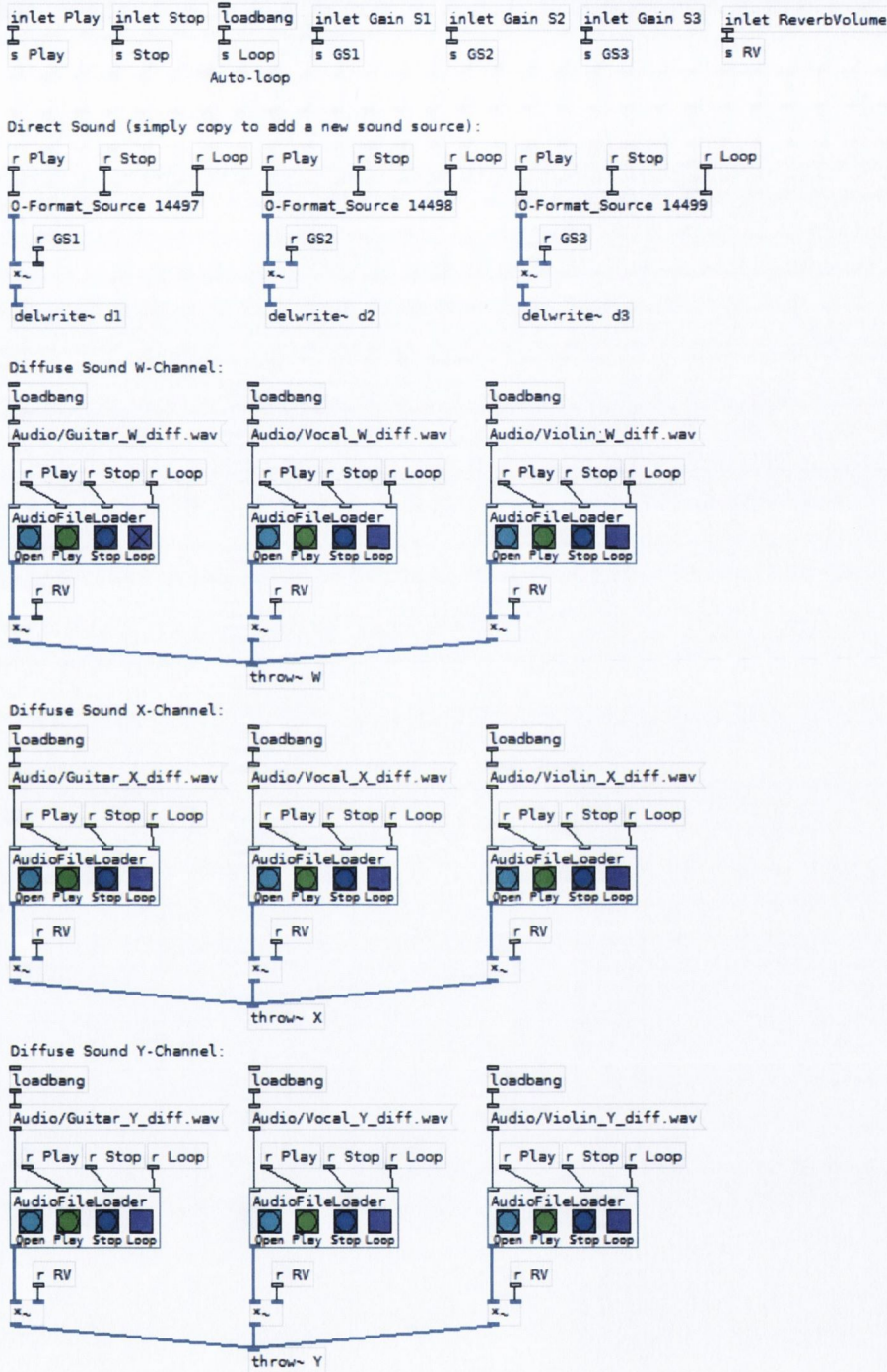
Figure 4.13: Audio_Assets abstraction which loads all the required sound files, performs the O-Format source decodes and routes the audio streams into relevant locations for further processing.
