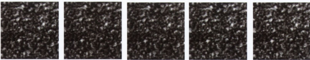
Figure 5. Five sequential speckle frames taken 2 ms apart, using an integration time of 2 ms and using a plastic target on the simulator. The simulator was running at 80 Hz, 197 \mu\text{rad} peak-to-peak.
