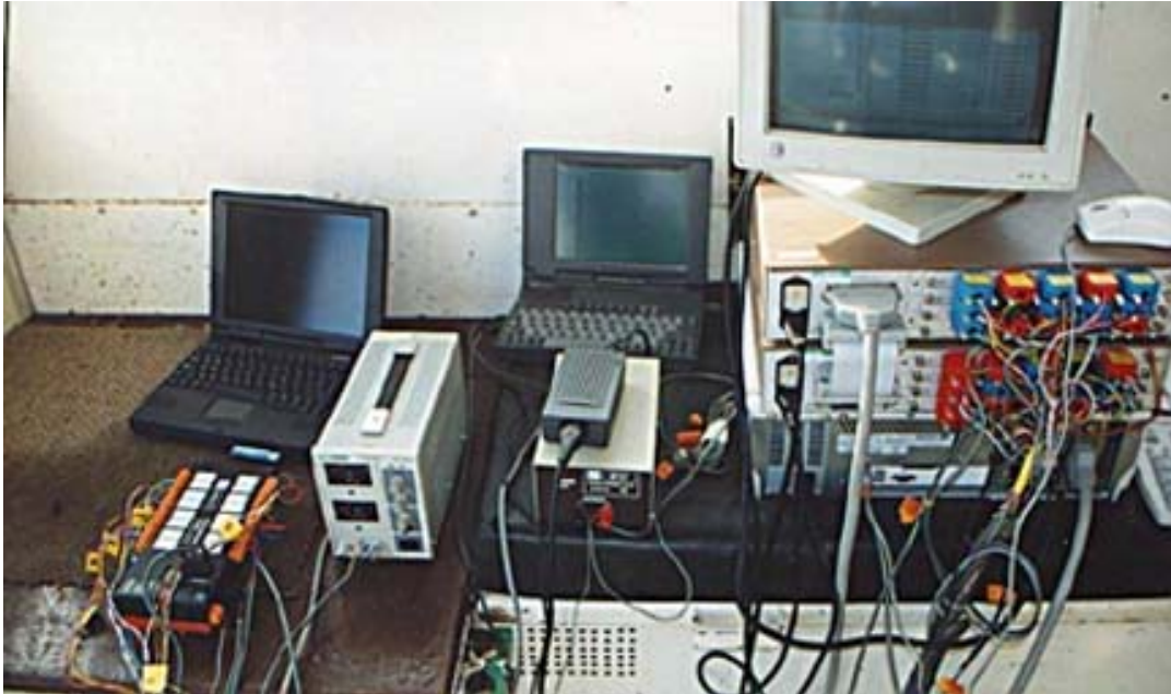
Figure 4-15 Data acquisition for pile tests
