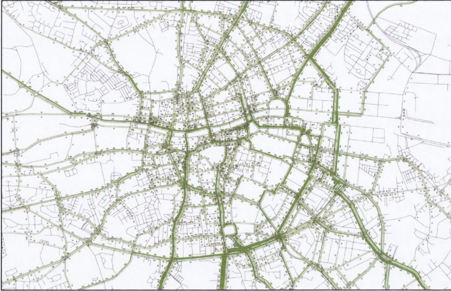
Figure 7.1 Bicycle traffic flow results from the NTA trip assignment model for Dublin city.
