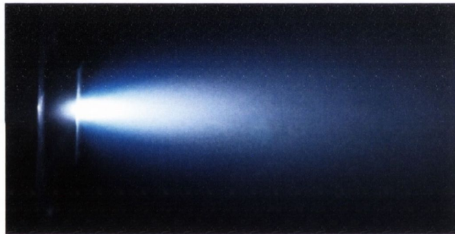
Figure 1.1: Time integrated image of a zinc plasma plume produced by a 1064 nm Nd:YAG nanosecond laser with an average fluence of 4 \text{ J cm}^{-2} .
