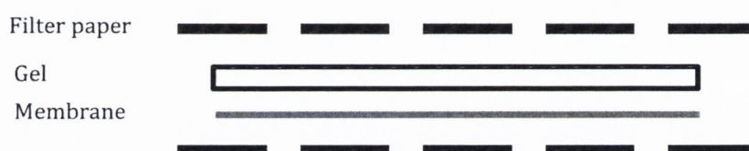
Figure 2.3 Filter paper, gel and nitrocellulose membrane sandwich (cross section).
