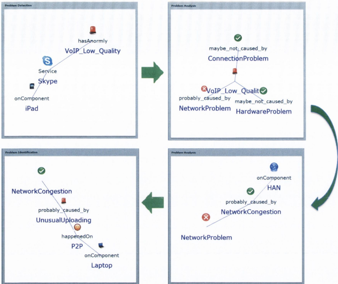
Figure 4-5 Analytic View: troubleshooting network problems
