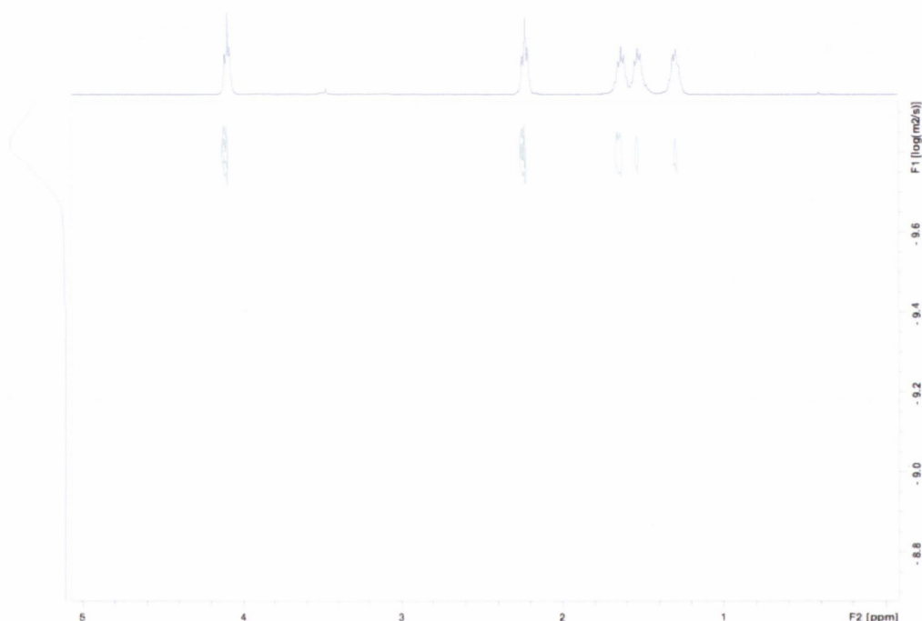
Figure 4.7: The DOSY spectrum of polycaprolactone in C_6D_6 . The F1 value is 9.77, corresponding to a value for the hydrodynamic radius of 33.90 Å ( c = 4 ) at 25 °C.
