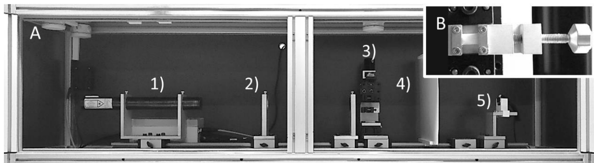
Figure 2 – (A) SALS setup consisting of 1) an unpolarised 5mW HeNe laser, 2) focusing lens, 3) automated sample positioner, 4) scatter plate and 5) CMOS camera, with (B) custom stretching device inset.
