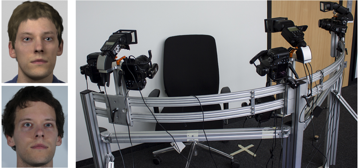
Figure 3.14: Our face scanning setup (right) and comparison between photographs and virtual reconstructions of our actor (left).
