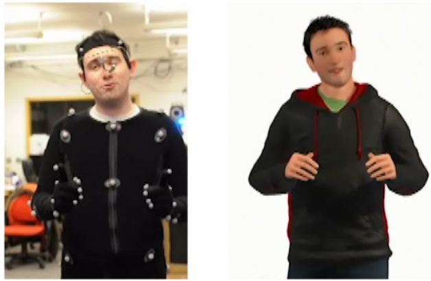
Figure 4.2: Actor during the capture session while portraying personality traits ( left ) and his motion applied to a virtual character ( right ).
