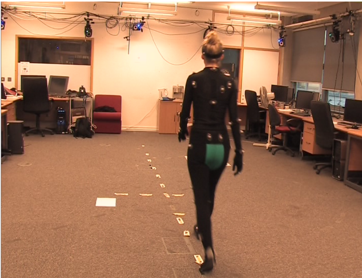
Figure 2.8: Motion capture setup at Graphics, Vison and Visualisation group at Trinity College Dublin. The actor is walking in the motion capture area, wearing a tight-fitting suit with reflective markers. The motion is recorded with Vicon optical mocap system of cameras, arranged circularly around the capture area.
