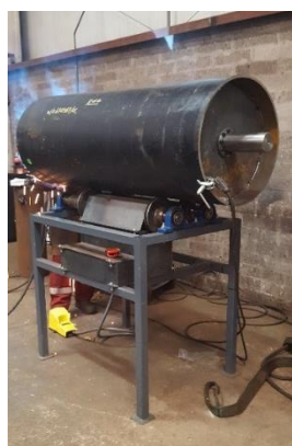
Figure 8 internally manufactured welding jig
