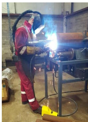
Figure 9 Welding jig in action
