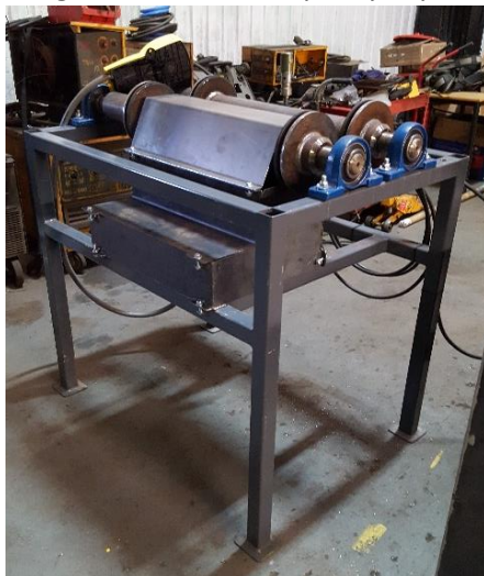
Figure 8 internally manufactured welding jig
