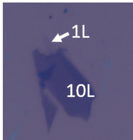
Figure B.2: Optical image of single and ten layer MoS 2 on a 300 nm SiO 2 layer on Si.
