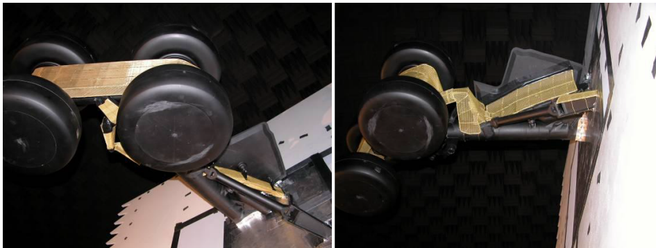
Figure 1.7: Mesh undertray and mesh leg door filler fairing and torque link fairing on a 1/4 scale model two wheel landing gear.[7]
