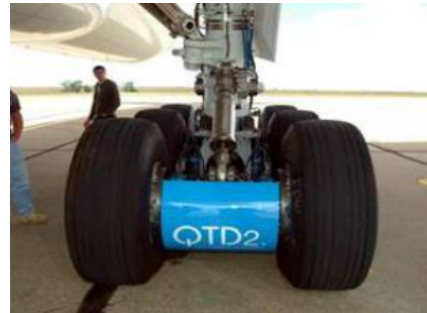
(b) Installed Toboggan Fairing
