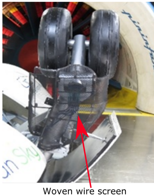
Figure 2.16: ALLEGRA Wire mesh screen installed on an MLG [16]
