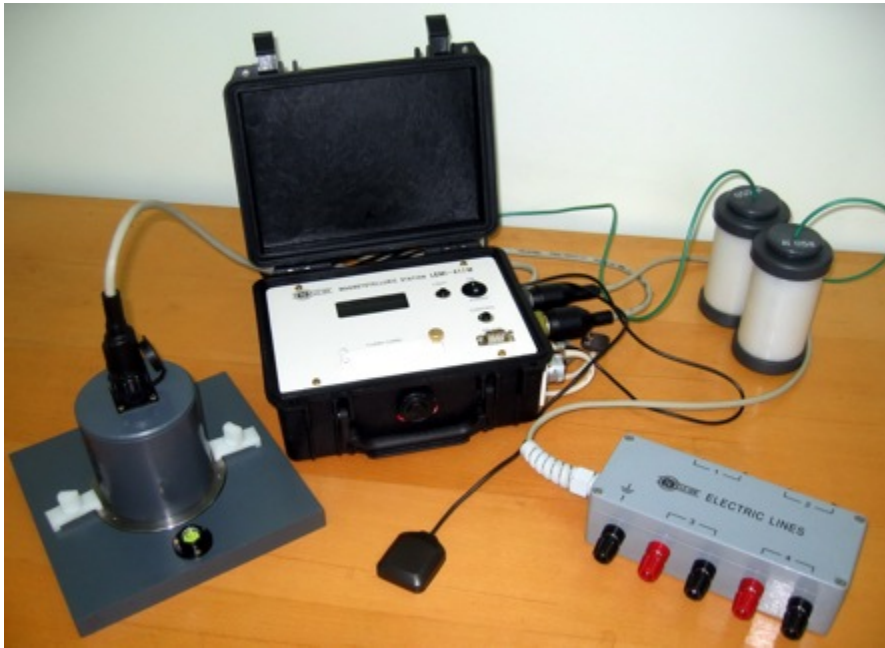
Figure 3.5: The 3rd generation LEMI-417M kit. Fluxgate magnetometer is left, recording device centre, and electrodes background right. Foreground right is the module to connect electrodes to the data logger. The electrodes in this picture (background right) are filled with a copper sulphide solution, rather than the lead-chloride electrodes used in this study. From www.isr.lviv.ua/lemi417.htm .
