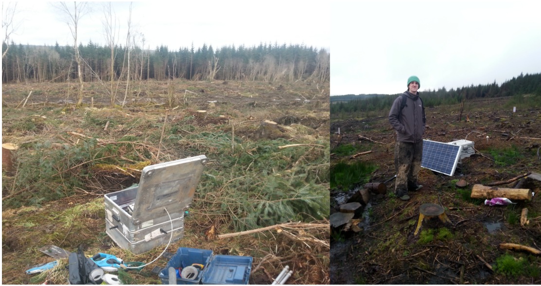
Figure 3.9: Left: site in Leitrim near Lough Allen. The broken terrain prevented electric-field cables from being buried. Right: the author at the Sligo site. The solar panel can be seen facing South to capture the Sun in Sligo.
