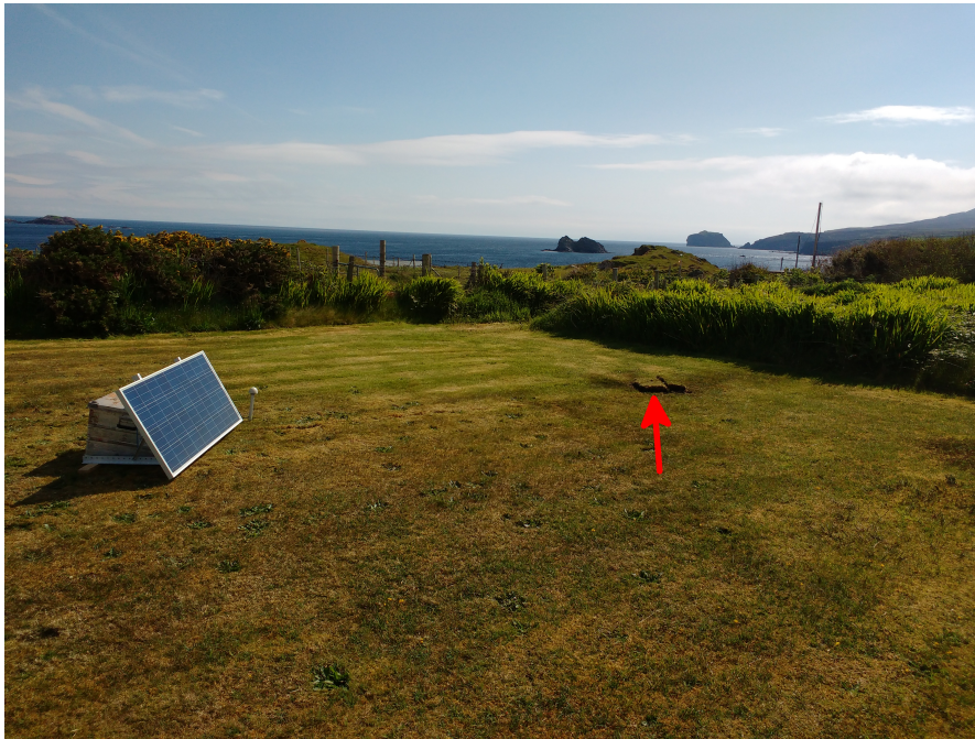
Figure 3.10: The Malin Head magnetometer site at the northernmost tip of Ireland. To the left is the solar panel and GPS receiver. To the right, beneath the cut earth, is where the magnetometer is buried (indicated with a red arrow).
