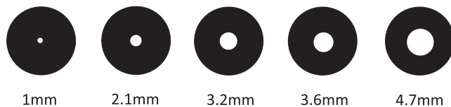
FIGURE 1. Scaled schematic diagrams of the tinted artificial pupil contact lenses used in our study.
