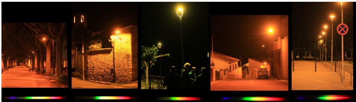
Figure 51: Tremp, Rambla Dr. Pearson (PC amber), Guardia de Noguera (amber filtered LED), Guardia de Noguera (green-yellow filtered LED), Les Avellanes (PC amber), Banyoles (PC amber Ignialight). Spectra obtained through a transmission grating (Astromedia, 1000 lines/mm) in front of a 30mm lens + Canon 550D camera.
