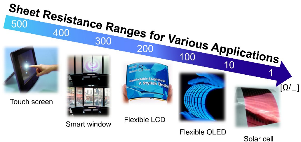
FIGURE 1.3. A schematic of the resistance ranges required for each potential application of metallic nanowire networks as transparent conductors. Adapted from Bae et al. [74]
