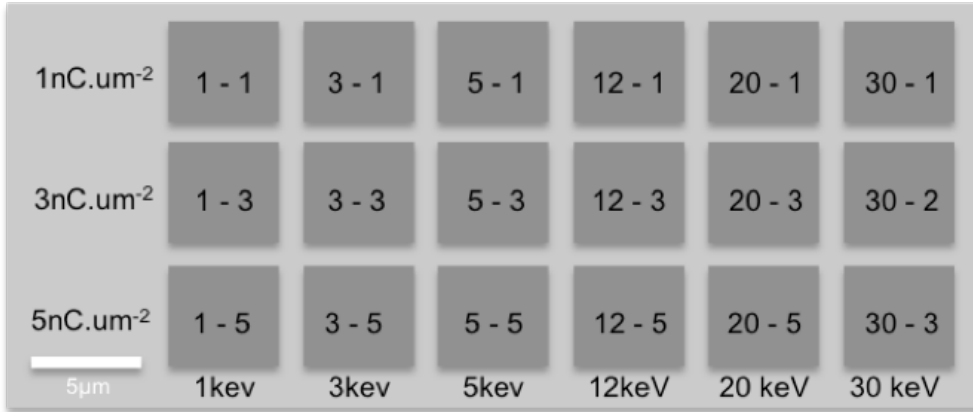
FIGURE 4.2: Irradiation array for the carbon layer deposition experiment.
