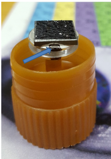
FIGURE 5.54: The HOPG test specimen affixed to an Al SEM stub. The marking on the stub, indicated by the blue arrow, was used to indicate the direction of ex-foliation after surface cleaving.
