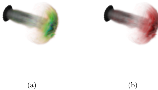
Figure 6.7: (a) Smoke density as variable X and gradient magnitude as variable Y at frame 160. Hue is X(i) , a=10 and b=5 ; (b) Hue is red. Note how parts of the smoke are desaturated and darkened based on the volatility and gradient magnitude
