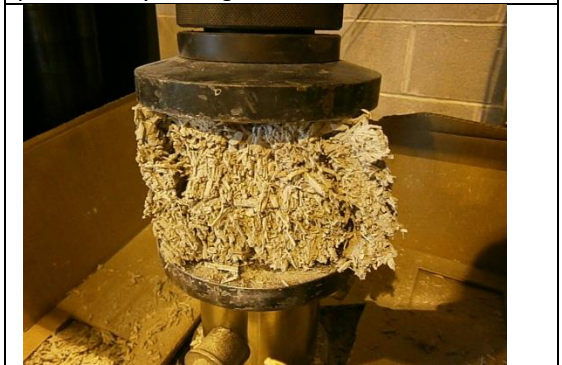
Figure 2. Failure of the concrete under axial load.
