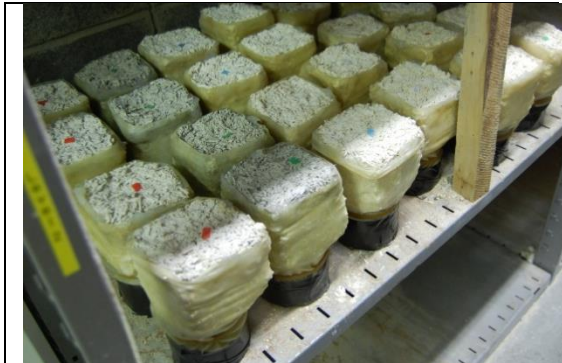
Figure 1. Hemp concrete undergoing permeability testing.
