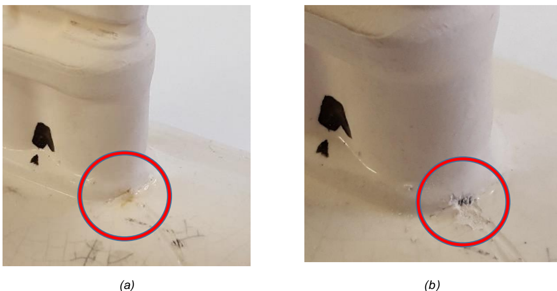
Figure 4.1-32 Failed FTEL IR element
