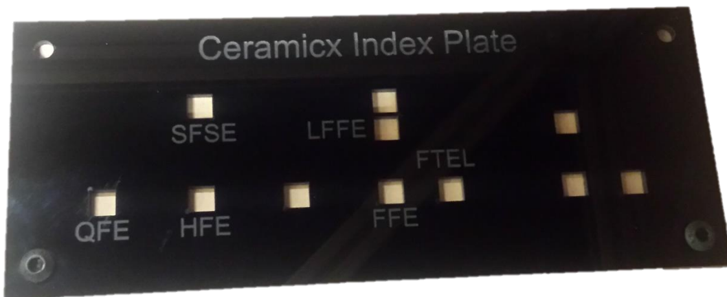
Figure 4.3-5 Indexing plate used to maintain IR element distance from camera
