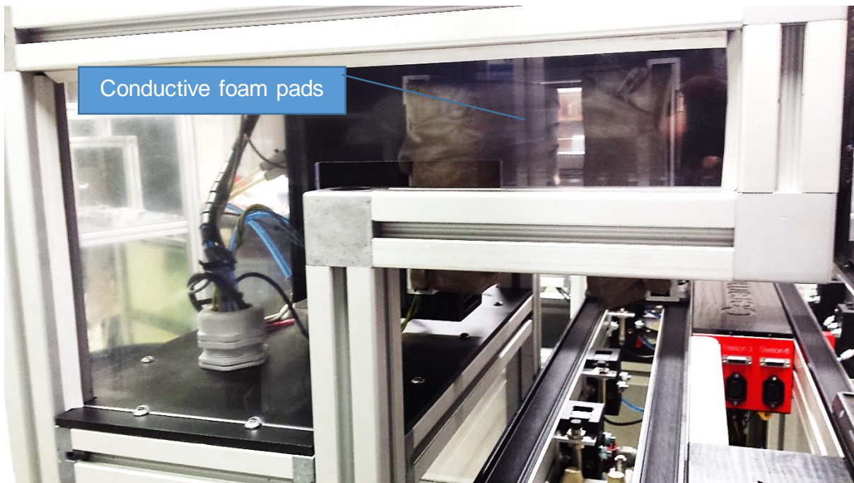
Figure 3.3-8 Test station 1 hipot test system
