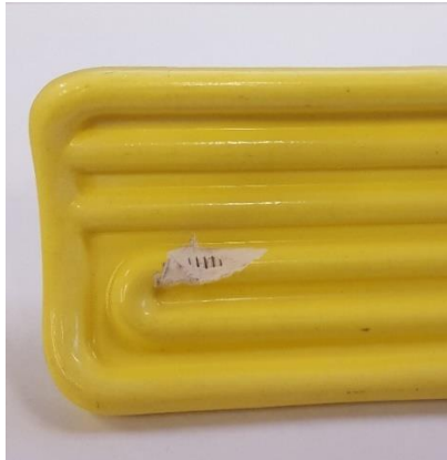
Figure 4.1-31 Chipped 500W FTE IR element
