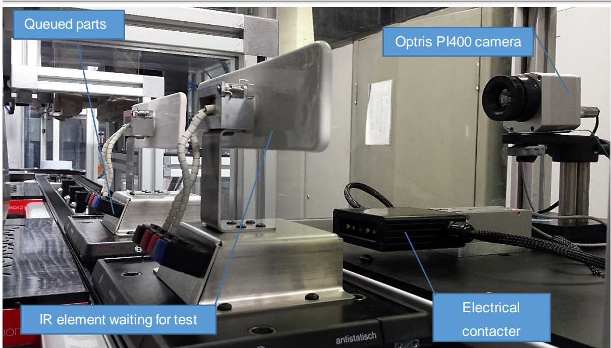
Figure 3.3-9 Part waiting for test station 2 thermal camera test
