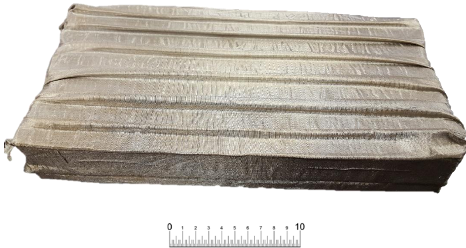
Figure 4.1-4 Image of pleated conductive fabric wrapped on foam pad with scale bar (cm)
