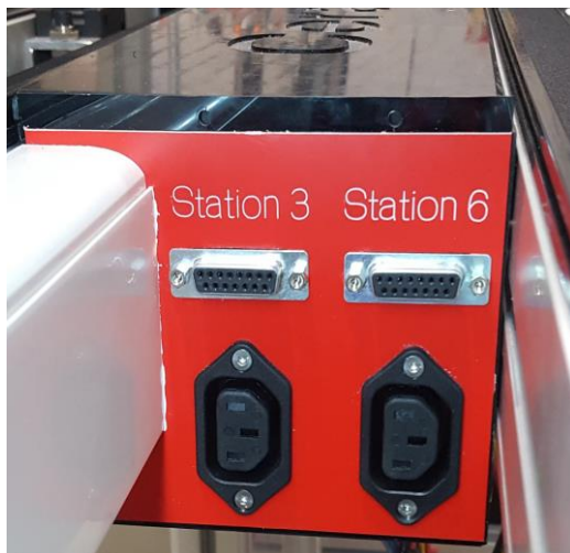
Figure 3.3-3 (a) Test station power and I/O socket
