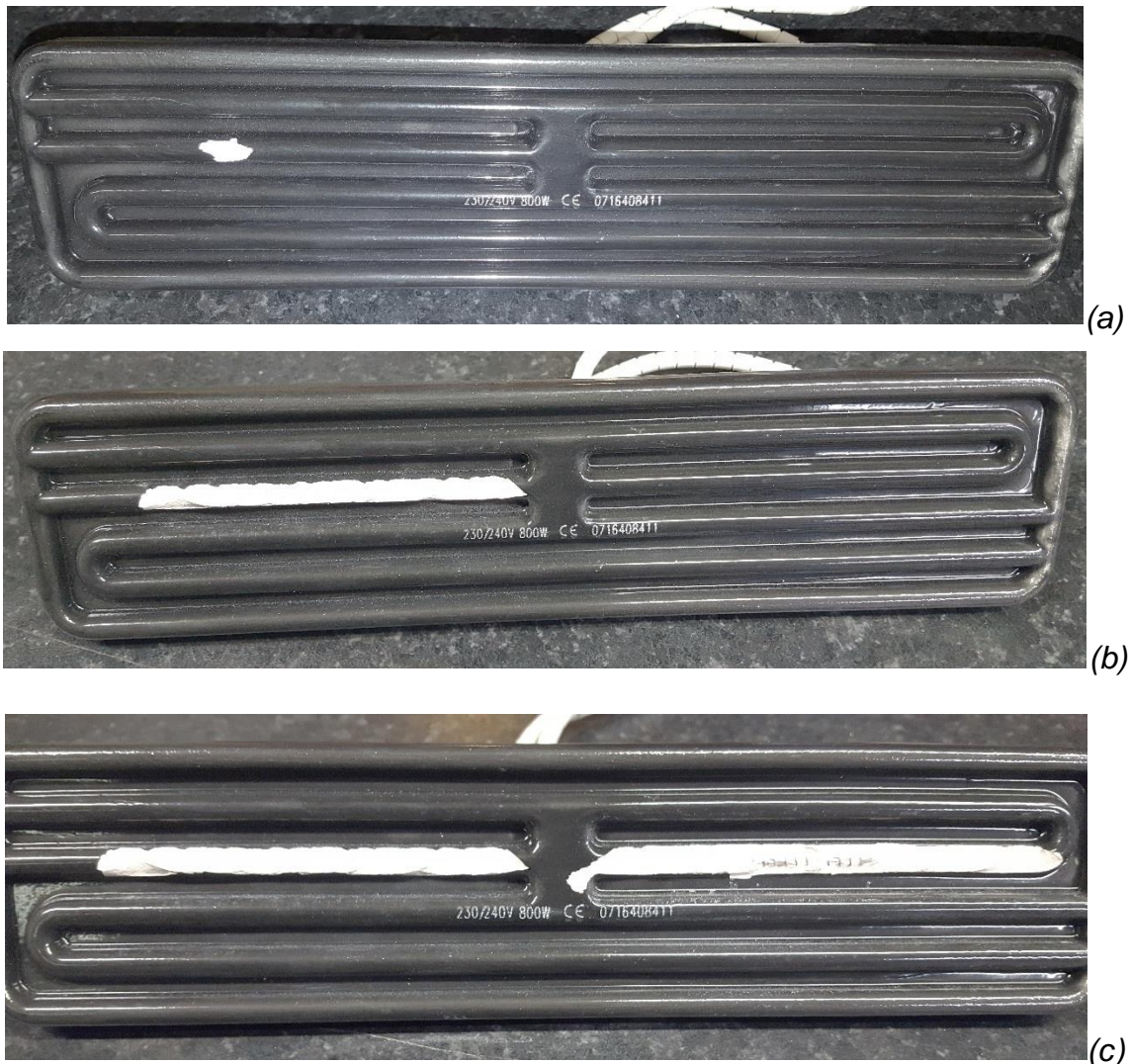
Figure 4.1-30 Scraping successive portions of glaze from 800W FFEH IR element
