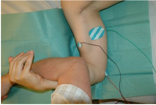
Figure 3.5: Electrode placement and counter resistance provided by the examiner's hand during SIP recording for Biceps Brachii (BB) muscle.
