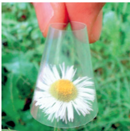
Figure 2.11: Flexible BCN-acrylic composite with 60% nanofiber content. Reproduced from Yano et al. [103]
