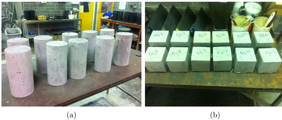
Figure 6.2.: (a) 10 concrete cylinders cast for Young's Modulus testing; (b) 12 concrete cube specimens cast for strength testing.
