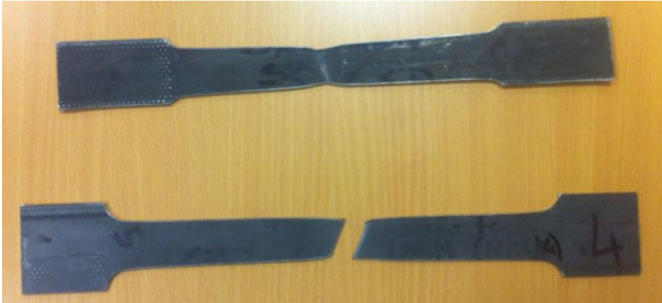
Figure 4.8.: Tensile Testing; Steel Coupons tested
