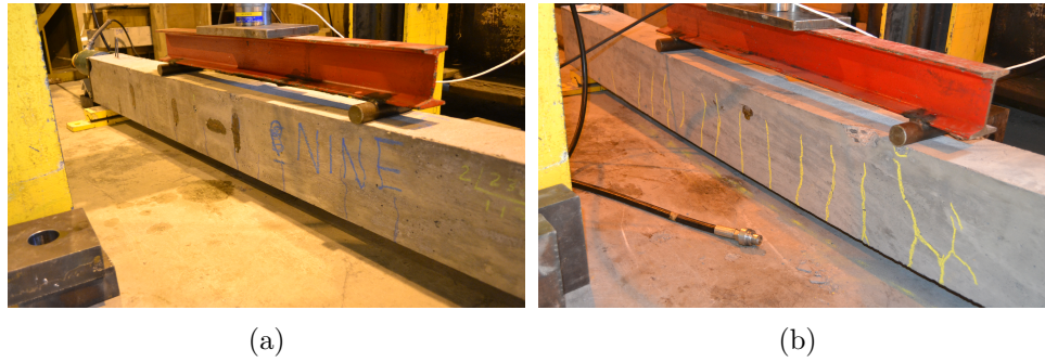
Figure 7.2.: Four Point Bending test; (a) Set-up in lab; (b) Cracked concrete beam
