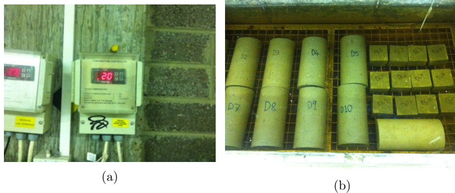
Figure 6.3.: (a) Concrete specimens stored in curing tank at 20^{\circ}\text{C} for a further 23 days; (b) Cubes and cylinders stored in the curing tank
