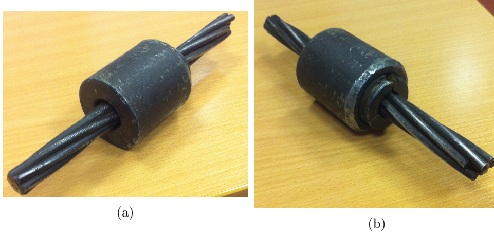
Figure 6.11.: Freyssinet 7-wire 15.7mm concentric strand and pre-stressing collet for anchorage
