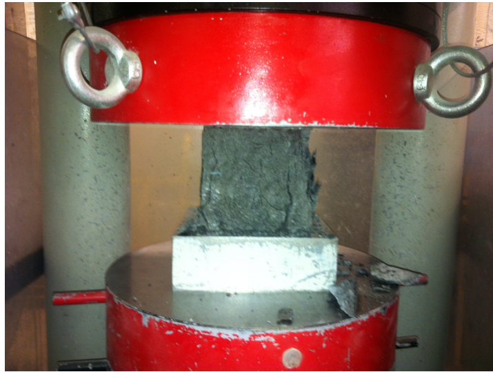
Figure 6.1.: Compression testing of concrete cube specimens
