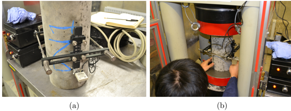
Figure 6.6.: Young's Modulus test set-up; (a) Extensometer placed on cylinder specimen (b) Cylinder loaded into compression testing machine
