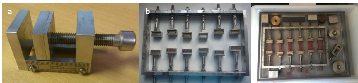
Figure 5.2-Compressive vice (a) and tensile rig (b) used for controlled muscle deformation. Samples loaded in the tensile rig for deformed(c).
