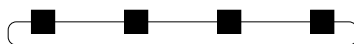
Figure 5.1: 1D torus, or ringlet, topology. Each node has one input and one output.
