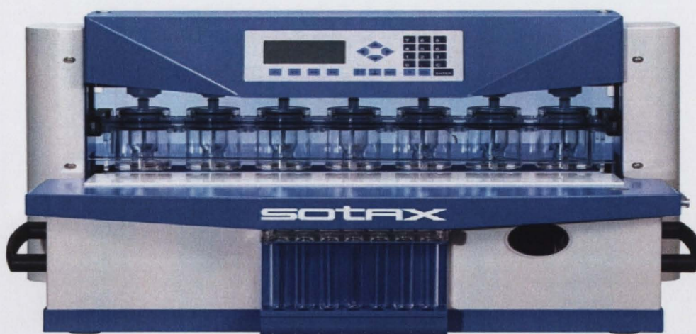
Fig 1.3 Flow through apparatus used for dissolution testing (Sotax online information sources)
