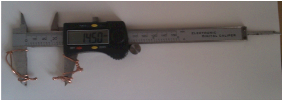
Figure 2.8. Vernier callipers, modified with copper wire, used to measure shell thickness.
