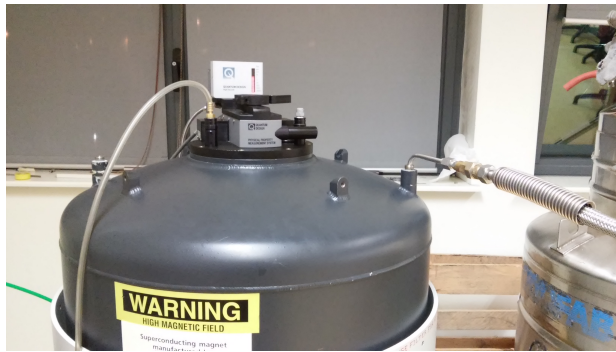
(a) The helium gas is connected to one of the transfer ports, the other one is blanked.
