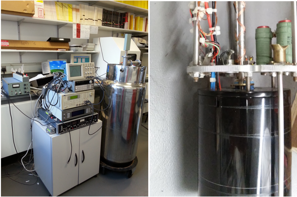
(a) Old SQUID setup with the pre-amplifier in a separate dewar. (b) New SQUID setup with the PCAR probe and the SQUID chip in the same dewar.
