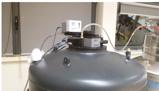
(a) The He gas line is swapped to the He supply dewar.
