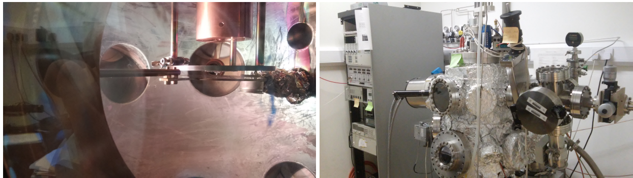
(a) Inside view of the organic deposition chamber.
