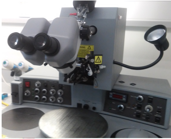
Figure 2.11: Picture of the wire bonder used for bonding of the \text{Mn}_2\text{Ru}_x\text{Ga} -based magnetic tunnel junctions.
