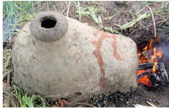
Figure 2.37: The kiln after the modifications made on its flue and stonion. Holes were also opened on the sides for allowing larger amounts of oxygen to flow during firing.
