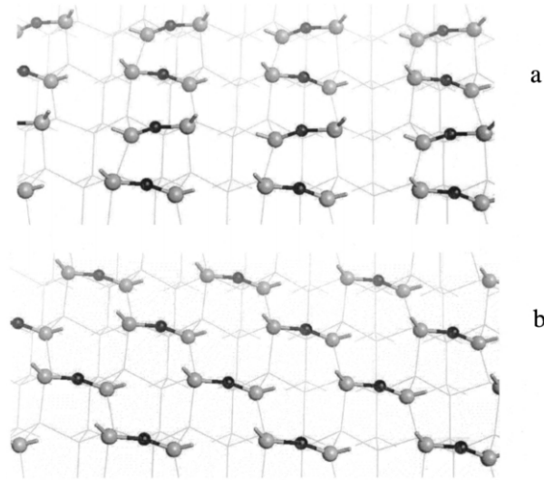
Figure 3.4: Row-patterned (a) and checkerboard-patterned (b) oxidation of a (001) Si surface as reported by Buczko et al [86]
