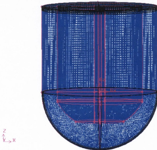
Figure 2.16 GAMBIT graphical interface illustrating the grid of the complete volume after meshing using the ‘Cooper’ scheme.
