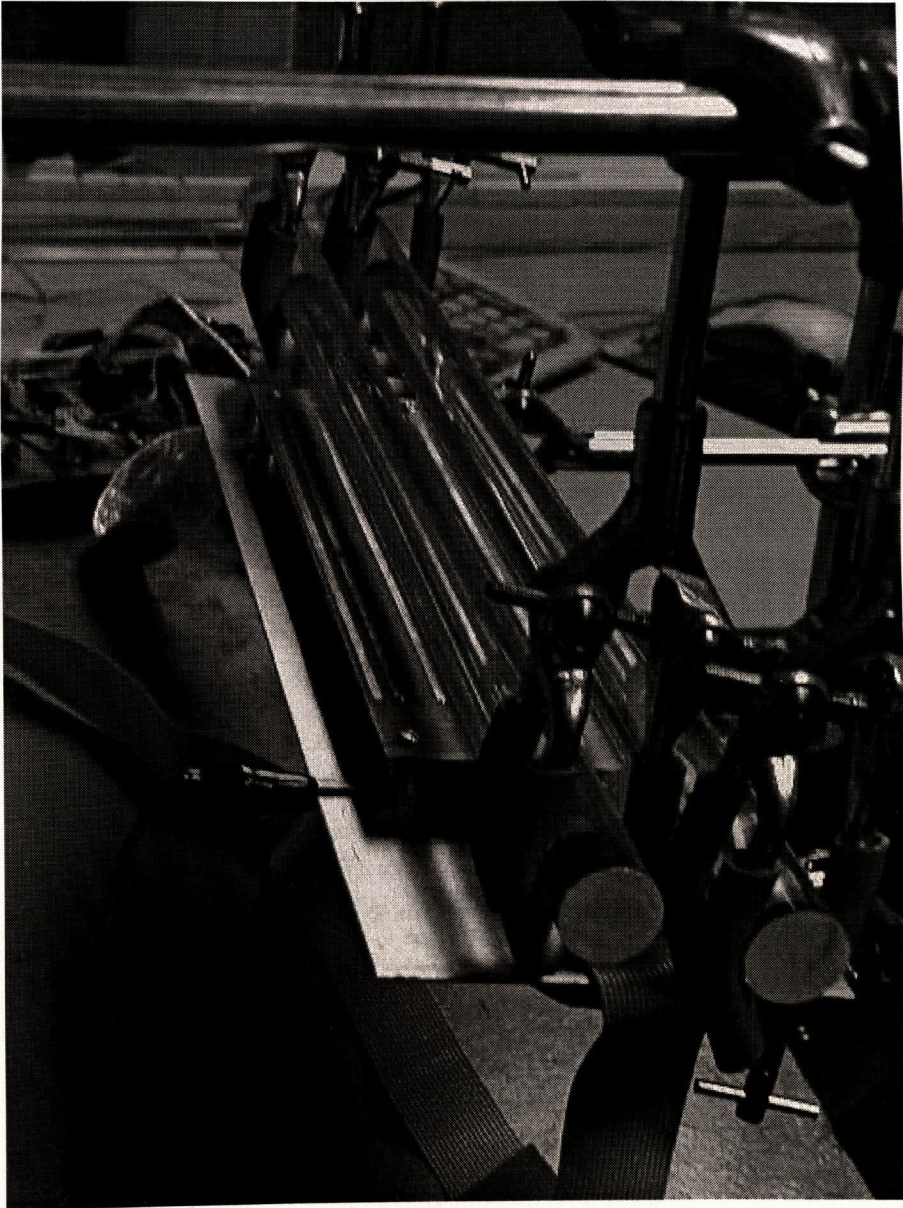
Figure 7.5: Two dielectric cylinders of radius 2cm and dielectric permittivity \epsilon = 3.7 in electrostatic field.
