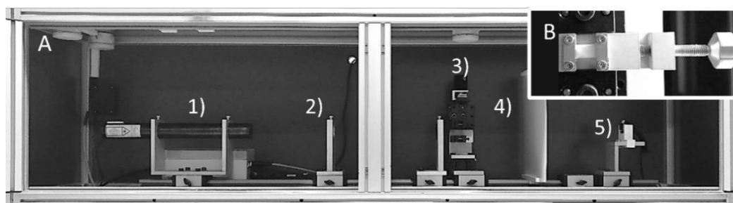
Figure 3.2 - (A) SALS setup consisting of 1) an unpolarised 5mW HeNe laser, 2) focusing lens, 3) automated sample positioner, 4) scatter plate and 5) CMOS camera, with (B) custom stretching device inset.
